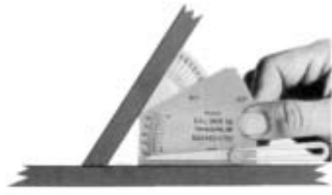
Checking Angle of Vertical Member
